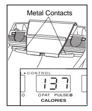
**moving your hands**. When your pulse is detected, the Pulse indicator will light, one or two dashes (--) will appear in the Calories/Pulse display, and then your heart rate will be shown. For the most accurate heart rate reading, continue to hold the contacts for about 15 seconds.
